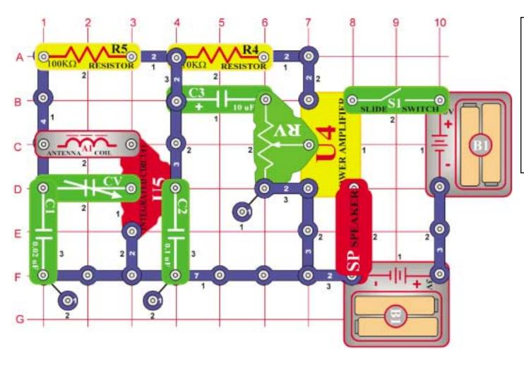
When you close the slide switch (S1), the integrated circuit (U5) should amplify and detect the AM radio waves all around you. The variable capacitor (VC) can be tuned to the desirable station. Varying the adjustable resistor (RV) will make the audio louder or softer. The power amplifier (U4) drives the speaker (SP) to complete the AM radio project.
