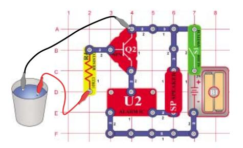
OBJECTIVE: To sound an alarm when water is
