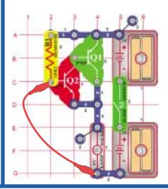
This light alarm circuit uses two (2) transistors and both sets of batteries. Build the circuit with the jumper connected as shown, and turn it on. Nothing happens. Break the jumper connection and the light turns on. You could replace the jumper with a longer wire and run it across a doorway to signal an alarm when someone enters.
