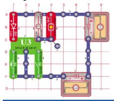
Build the circuit shown on the left. Activate the circuit by flipping the switch or pressing the press switch (S2), do both several times and in combination. You will hear exciting sounds and see flashing lights, as if a space battle is raging!
