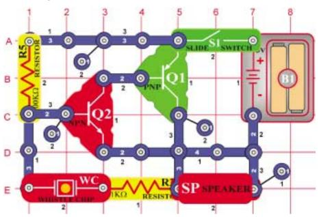
Build the circuit and turn it on, you hear a high-frequency sound.
