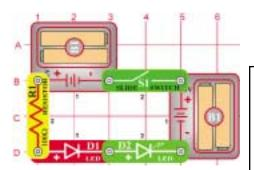
Put on the switch and the two LEDs will have the same brightness. When connected in series, all components will have equal electric current through them.
