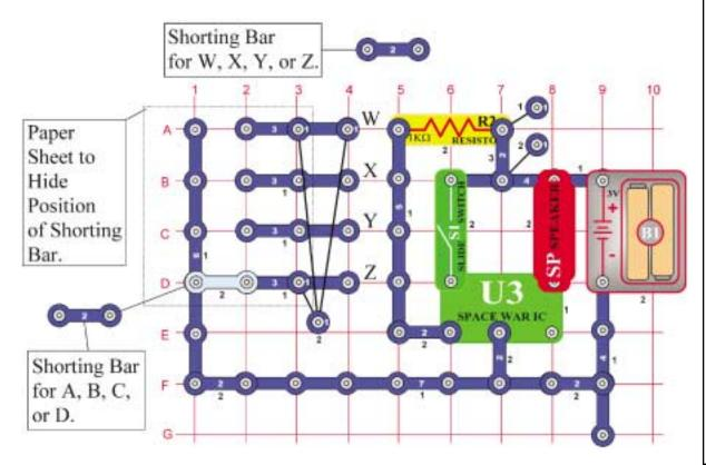
Build the circuit shown on the left. It uses two (2) 2-snap wires as shorting bars.
