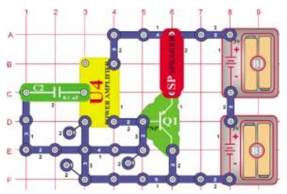
The tone you hear is the frequency of the oscillator. Install different values of capacitors in place of the  $0.1\mu F$  (C2) to change the frequency.
