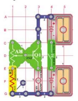
OBJECTIVE: To demonstrate adjusting the gain of a transistor
