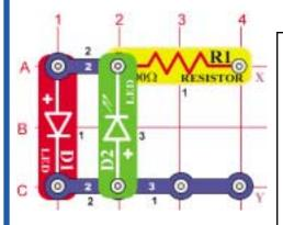
Use this circuit to check the polarity of a battery. Connect your battery to X and Y on the drawing using the jumper cables (your 3V battery pack (B1) can also be snapped on directly instead). If the positive (+) side of your battery is connected to X, then the red LED will be on, if the negative (-) side is connected to X then the green diode will be on.
