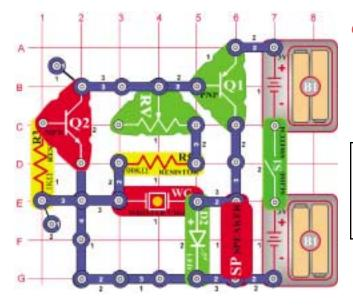
Build the circuit, turn it on, and move the setting on the adjustable resistor. It makes a loud, annoying whine sound. The green LED (D2) appears be on, but it is actually flashing at a very fast rate.
