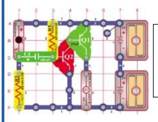
Install the parts. The lamp (L1) will be on. It will be off as long as you blow on the mic (X1). Speaking loud into the mic will change the brightness of the lamp.
