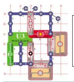
Place the fan onto the motor. Space war sounds are heard if light shines on the photosensitive resistor OR if you press the press switch (S2), the fan may start to spin, but will only get to high speed if you do BOTH. Try various combinations of shining light and holding down the press switch.
