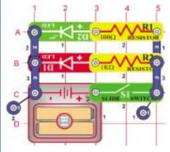
Put on the switch and notice the difference in brightness between the two LEDs, this comes from the difference of their in-series resistance. The smaller the resistance, the stronger the electric current that is allowed to pass through. This is how resistance limits the current.
