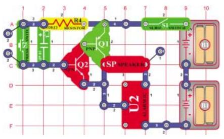
Turn on the switch, then press and release the press switch. You hear a siren that slowly fades away and eventually goes off. You can modify this circuit to make machine gun or ambulance sound instead like in the other projects. You can also replace the  $10\mu F$  capacitor (C3) with the  $100\mu F$  (C4) or  $0.1\mu F$  (C2) to greatly slow down or speed up the fading.
