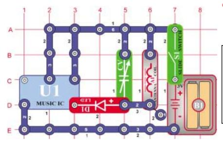
You need an AM radio for this project. Build the circuit shown on the left and turn on the switch. Place it next to your AM radio and tune the radio frequency to where no other station is transmitting.
