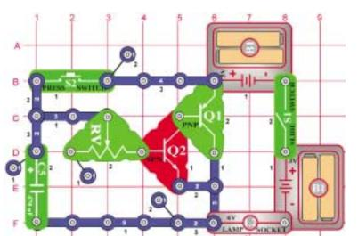
Be sure to use the 6V lamp (L2) for this circuit. Turn on the switch and press the press switch (S2). The lamp stays on for a few seconds after you release the press switch. You can change the delay time with the adjustable resistor (RV).
