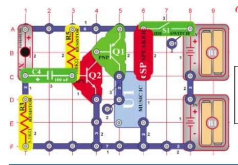
Build the circuit and turn it on, music plays. Since it is loud and annoying, try to shut it off by blowing into the microphone (X1). Blowing hard into the microphone stops the music, and then it starts again.
