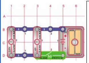
Turn on the slide switch (S1) and both lamps will light. If one of the bulbs is broken then the other will still be on, because the lamps are in parallel. An example of this is most of the lights in your house; if a bulb is broken on one lamp then the other lamps are not affected.
