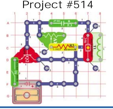
0 2 Build the circuit and set the variable resistor (RV) control all the way to the right. Turn on the switch (S1) and you hear a sound like a faucet dripping. You can speed up the dripping by moving the variable resistor control around.
