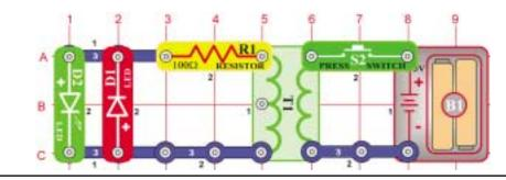
Watch the LEDs (D1 and D2) as you press or release the switch (S2). The red LED (D1) lights briefly just as you press the switch and the green LED (D2) lights briefly just after you release it, but neither lights while vou hold the switch down. Why?
