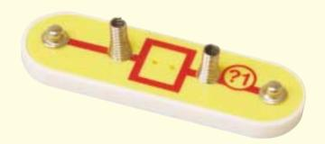
The two-spring socket (?1) just has two springs, and won't do anything by itself. It is not used in any of the experiments. It was included to make it easy to connect other electronic components to your Snap Circuits. It should only be used by advanced users who are creating their own circuits.
