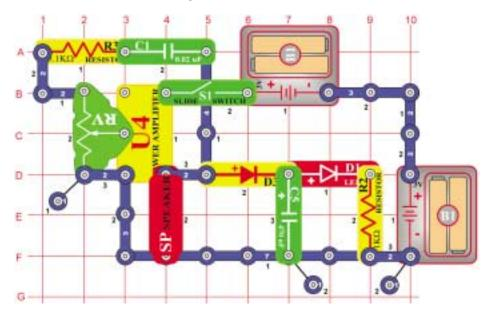
This circuit is based on the Trombone project #238. Turn on the switch (S1) and set the variable resistor (RV) for mid-range for the best sound. The LED (D1) will also be lit.
