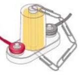
An electric current flowing in a coil of wire has a magnetic field, which tries to suck iron objects into its center. You can see this using the circuit from project #660.
