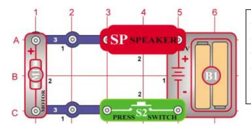
Place the fan on the motor (M1). Press the switch (S2) and listen to the motor. Why does the motor make sound?
