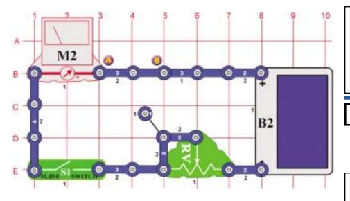
Place the circuit near a bright light and set the variable resistor (RV) so that the meter (M2) reads "10" on the 10MA setting. Now replace the 3-snap between points A and B with another component to test, such as a resistor, capacitor, motor, photoresistor, or lamp. The  $100\mu F$  (C4) or  $470\mu F$  (C5) capacitors will give a high reading that slowly drops to zero.
