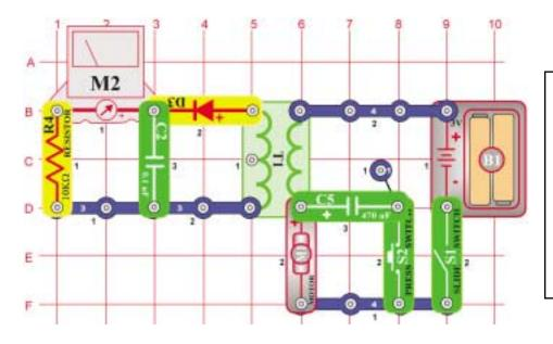
Set the meter (M2) to the 10MA scale. Place the fan on the motor (M1) and turn on the switch (S1), the meter measures the current on the other side of the transformer (T1).
