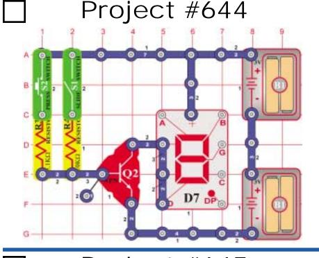
The NOR gate works the opposite of the OR. Using the chart set the switches to the different states. The display lights the letter "L" when either switch is turned on.
