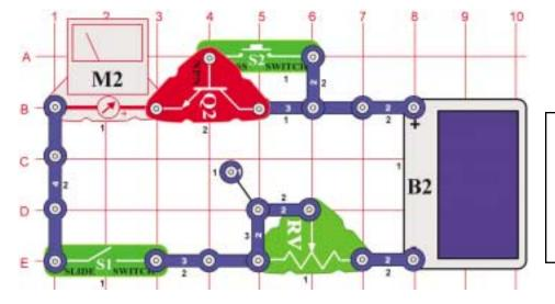
This circuit is just like the one in project #551, but tests the NPN transistor (Q2). The meter will read zero unless both switches (S1 and S2) are on, then the variable resistor (RV) sets the current. If you have the same light and RV setting as project #552 with the diode (D3), then the meter (M2) reading will be higher with the transistor.
