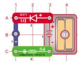
The vibration switch contains two separate contacts; a spring is connected to one of the contacts. A vibration causes the spring to move briefly shorting the two contacts. This simple circuit demonstrates how the vibration switch works. Build the circuit and the LED does not light. Tap the vibration switch or table and the LED lights for every tap. It acts like a temporary switch connecting the battery to the LED.
