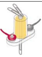
Snap two 2-snaps around a paperclip and lift them with the electromagnet, as shown here on the left.
